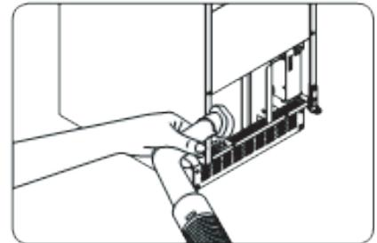
Reassemble the panel using the two screws to after cleaning
