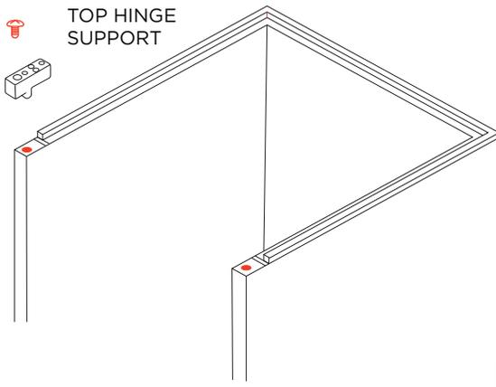
4. Remove the Top Hinge Support which is held in place by one (1) screw from the right hand side and transfer it to the left hand side re-attaching it with the screw.
